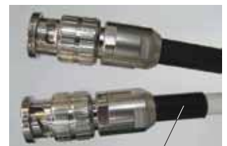
In multiple type case, confirm the shrinkable tube covered abt. 15mm or more.
